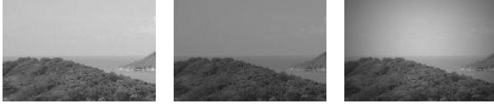
Figure 4. Original image (left). Image captured with a shorter exposure duration (middle). Image captured with heavy lens vignetting (right). Note that exposure duration difference produces the change of the global brightness, while lens vignetting darkens the image gradually when getting close to the corner.
