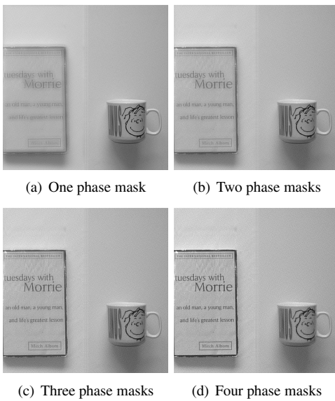
Figure 5. Reconstructed images with different numbers of phase masks incorporated.
