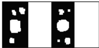
Fig. 4. Bright dots in black stripes are induced by multi-reflections and need be rectified.
