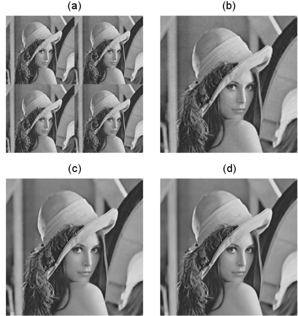
Figure 1. Comparisons between different HR reconstruction methods for the test image Lena : (a) LR noisy images, (b) IBP result, (c) LPR-RICl result, (d) SK-LPR-RICl result.
