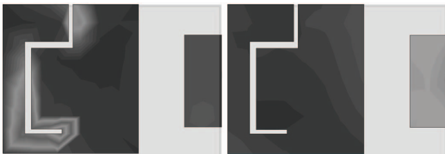
Figure 6. Electric & Magnetic Field Distributions for the BA^{right} geometry at f = 1.99 GHz . The field distributions are the same for both the BA^{right} and the BA^{left} geometries. On the left is the magnetic field distribution for the GSM antenna and on the right is the electric field distribution for the 3G/4G antenna. (Dark grey is zero field and lighter greys represent stronger field strength).
