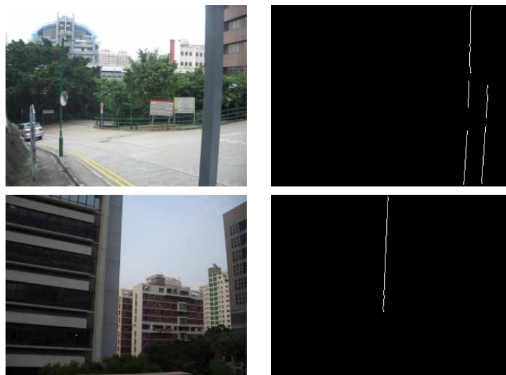
Fig. 8. Top: An example image from Casio and its edge map. Only a few short straight lines appeared in the edge map. Bottom: Another example image from Casio and its edge map. Only one straight line in the middle of the image. Lines which are short or at the center may not provide useful information for distortion estimation. The k_1 and k_2 values from both examples are far from the majority of Casio images in fig. 5.
