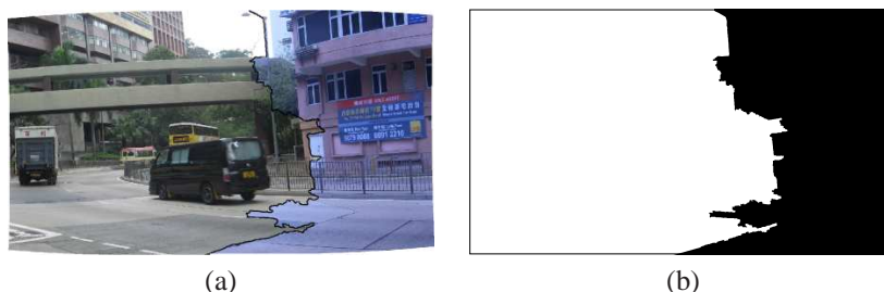
Fig. 3. (a) Result of pixel selection according to the curve generated by our method. No moving object is cut. (b) Binary mask \alpha(x,y) corresponds to the curve.
