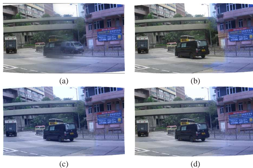
Fig. 4. Stitching Result of (a) Exposure Compensation, (b) Wavelet Blending, (c) Gradient Stitching and (d) Our method, assigning 1 to the middle 85% vertical portion of \beta_2(x, y) .
