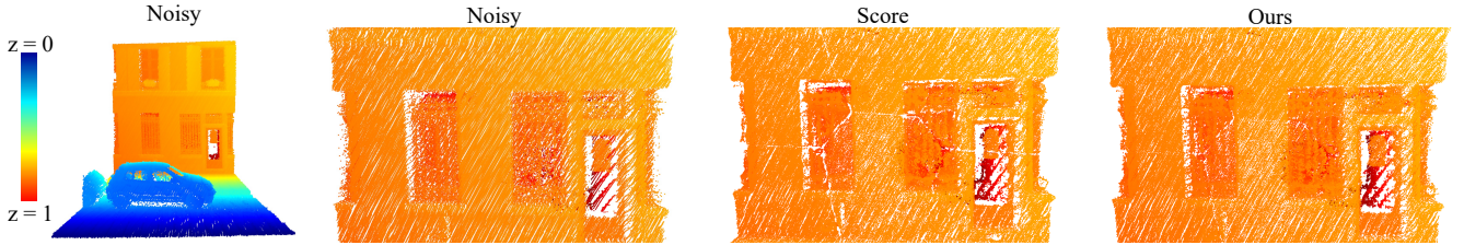
Fig. 6: Point cloud denoising comparisons on the real-world dataset Paris-rue-Madame [18]. The color of each 3D point varies according to its z coordinate (perpendicular to the plane).
