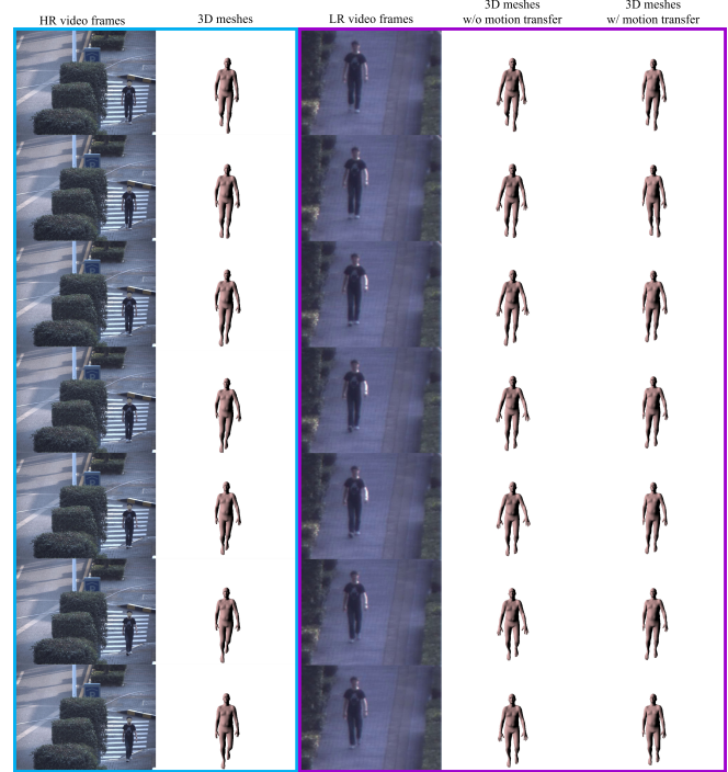
Fig. 8: Our motion transfer technique improves 3D human mesh reconstruction performance. In the LR video, we observed misaligned arm positions. However, the results with motion transfer effectively correct the human poses.
