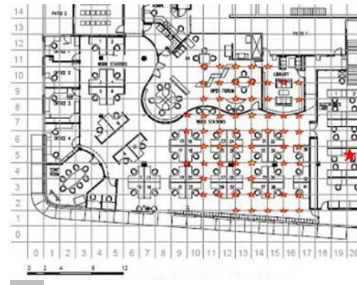
Fig. 11. Radio placements at the BWRC to measure gains from cooperative sensing
