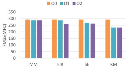
Fig. 10. Fmax of the accelerators generated using QuickDough
